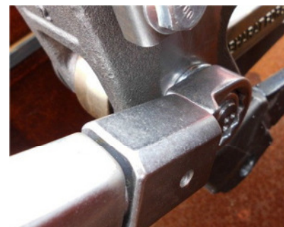
Fig. 3 Torque Wrench with insert
